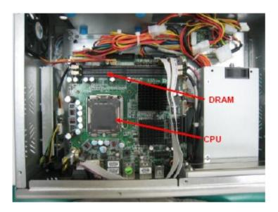
Step 3: Install the CPU and DDR DRAM in the PC 8120.
